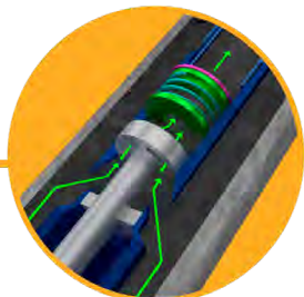
Bypass Valve (Open)
