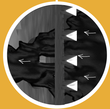
Fluid flowing through the top bypass valve
